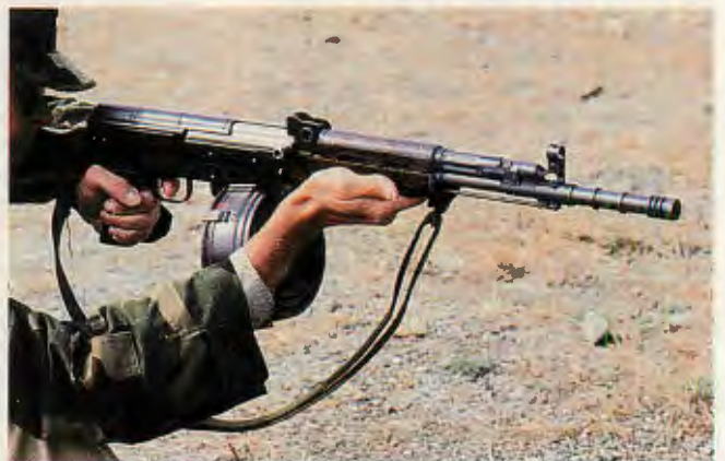
ABOVE LEFT: PLA officer adjusts electronic equipment used in SOF's test and evaluation of PRC military small arms. Digital readout indicates numerical value of score and location of impact on target. Weapon tested here is Type 81 assault rifle. ABOVE RIGHT: Firing the Type 81 rifle with 75-round drum.
